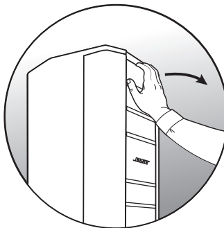
Pulling the array out
